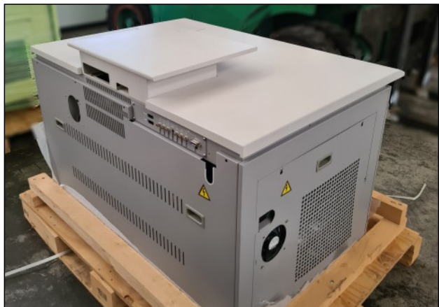
HV tank, video I/O
